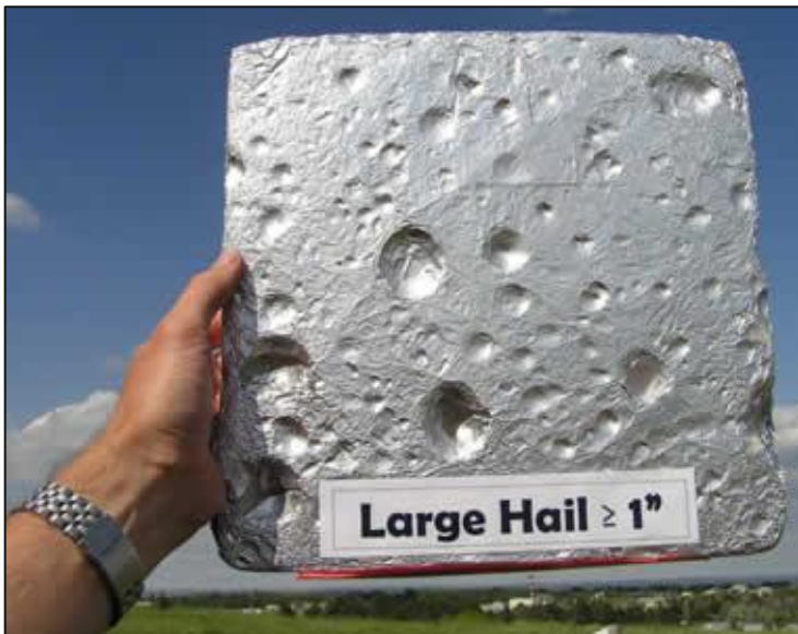
Figure 4. Dents in a hail pad after a severe hail event (Source: CoCoRaHS )
