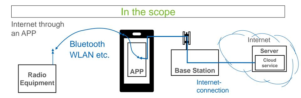
The Radio Equipment is capable to connect itself to the internet (Server)!
