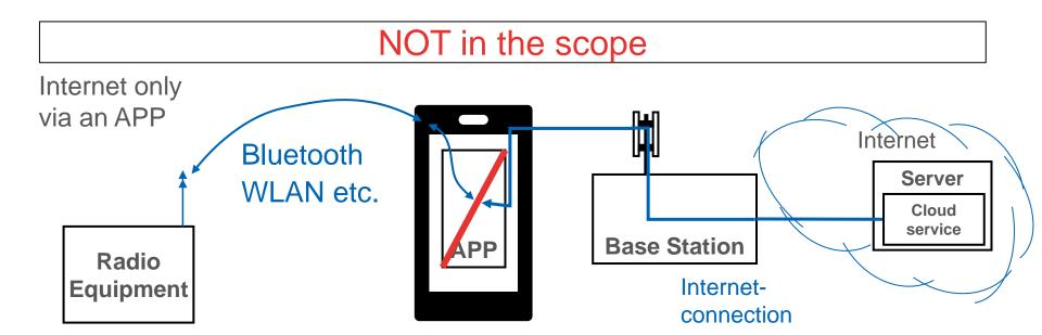
The Radio Equipment is not capable to connect itself to the internet!
